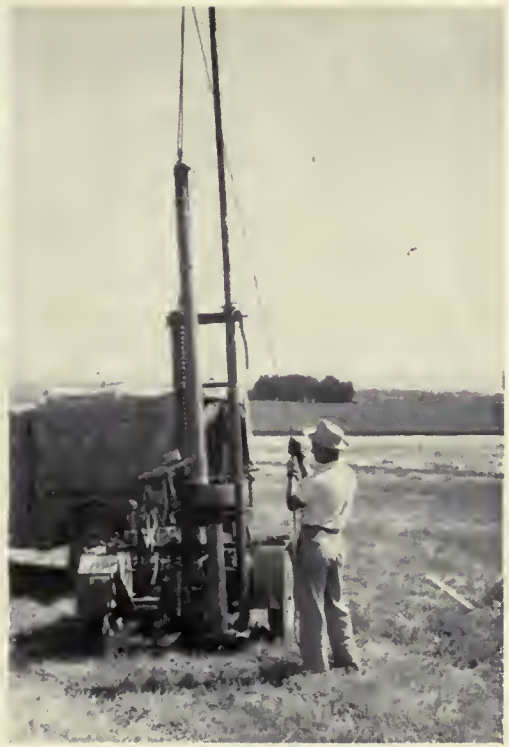
IN THE GROUND. —Special machines carve cylinders of undisturbed soil for analyses or to observe soil characteristics and permeability, especially in relation to drainage. Photo courtesy of Oregon State College.
